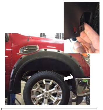
**STEP 8:** Install the provided U shape metal clip at the (1) remaining slot location in the Fender Flare. Ensure that positive pressure is applied on the Fender Flare to the vehicle fender when installing clips. Slide the clip over the Fender Flare and the inner lip of the front bumper fascia ensuring that the barb in the clip locates in the slot of the Fender Flare. Ensure that the rubber seal is flush neatly against the vehicle body.
