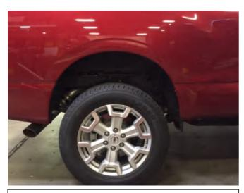
**STEP 9:** Clean the body area where the Fender Flares will make contact. Ensure fenders are dry prior to install. For models equipped with factory fender flares, removal of factory flares is required, please consult the vehicle service manual for factory fender flare removal.
