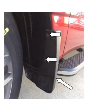
**STEP 5:** For vehicles equipped with factory mud gaurds. Remove (3) retaining screws to remove mud guard. Store mud guard in a safe place, it will not be re-used for Fender Flare installation. Reinstall screw in underside rocker panel area and retain (2) remaining screws from inner wheel arch for Fender Flare Installation.
