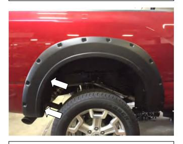
**STEP 12:** Place Fender Flare on vehicle, ensure the slots in the Fender Flare align with the holes in the wheel arch from the previously removed factory screws. Using #2 Phillips head screwdriver re-install the previously removed (2) screws through slots in Fender Flare.
