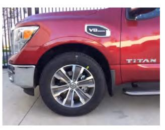
**STEP 4:** Clean the body areas where the Fender Flares will make contact. Ensure fenders are dry prior to install. Turning tires outward during install of each Fender Flare will ensure ease of install at bottom fixing points. For models equipped with factory fender flares, removal of factory flares is required, please consult the vehicle service manual for factory fender flare removal.
