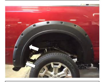
**STEP 11:** Place Fender Flare on the vehicle into the position of best fit. Note where (2) slots in rear of Fender Flare correspond with existing screws / fixing points in the wheel arch. Remove Fender Flare. Remove any existing vehicle screws in locations as shown with #2 Phillips head screwdriver. Maintain screws for re-installation.
