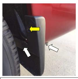
**STEP 10:** For vehicles equipped with factory mud gaurds. Remove (3) retaining screws to remove mud guard. Store mud guard in a safe place, it will not be reused for Fender Flare installation. Reinstall screws in underside rocker panel and innermost wheel arch area retain remaining uppermost screw for Fender Flare
